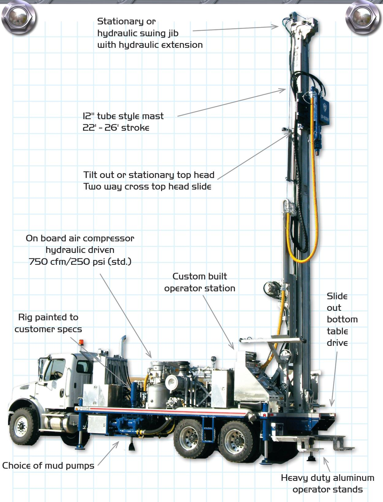
Stationary or hydraulic swing jib with hydraulic extension
